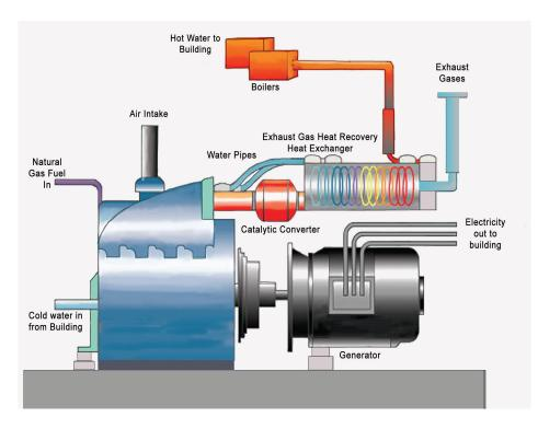
process the excess energy is wasted and exhausted out a chimney. Through cogeneration, the high-temperature combustion produces both hot water as well as electric power. The performance is
