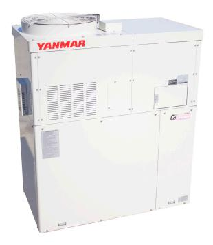
Using natural gas or propane, the CP10WN's high-efficiency generator provides 10kW of electrical power. The engine heat is captured and heats water at a rated temperature of 158°F for immediate use or storage in your facility. Excess electricity production may be sold back onto the grid in certain states, creating a credit on your electric bill.
