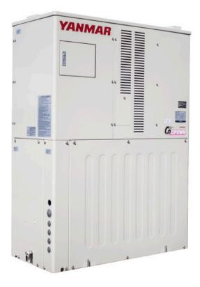
Using natural gas or propane, the CP5WN's high-efficiency generator provides 5kW of electrical power. The engine heat is captured and heats water at a rated temperature of 149°F for immediate use or storage in your facility. Excess electricity production may be sold back onto the grid in certain states, creating a credit on your electric bill.
